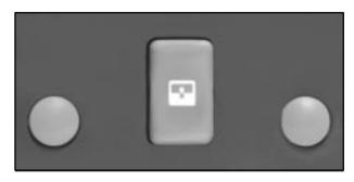
To open the sunroof and sunshade, press and hold the rear side of the button, located on the overhead console, until the sunroof reaches the desired position or until it stops at the built-in comfort position. The comfort position stops the sunroof from opening completely.
